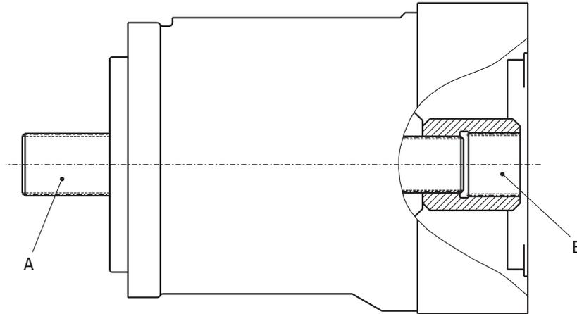
The diagram Torque transmission of HMF / A / V / R shows the output side (A) and the PTO through-shaft (B) of a motor.
