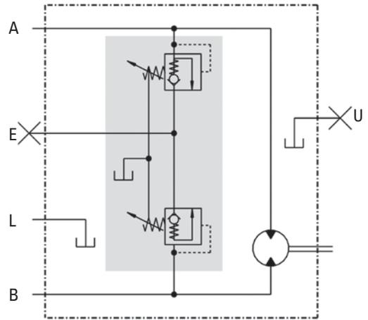
**With Dual Pressure Crossline Relief Valve Protection**
