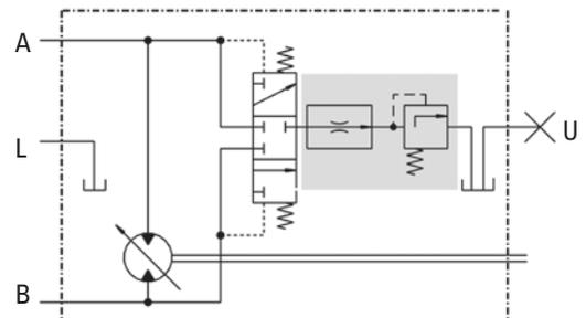
Flow-controlled purge flushing in an open loop circuit approx. 4 l/min at 5 bar set pressure (independent of low pressure) diagram 4
