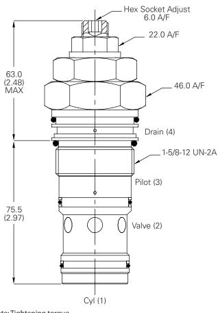
Note: Tightening torque of "F" adjuster locknut -20 to 25 Nm.
